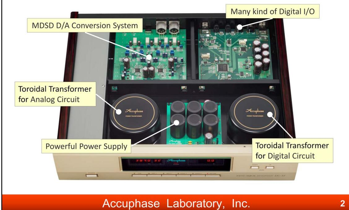
DC-37 has the construction which digital circuit and analog circuit including power transformers are completely separated.
